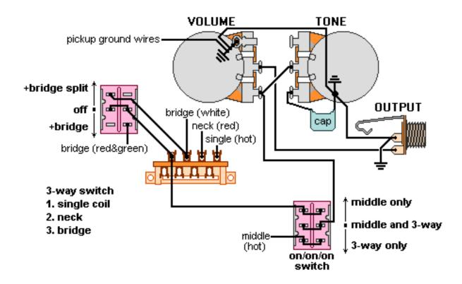
Bridge pickup selector can be on-on-on or on-off-on. Ground bridge pickup black& bare wires. Solder black & white from neck pickup together and tape connection. Ground green and bare wires. All other pickup wires not shown or mentioned go to ground.
