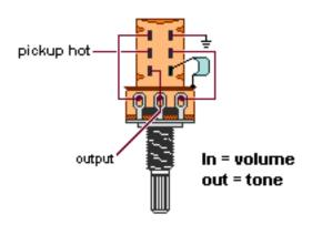
Note: Tailpiece should be connected to common ground. All grounds 🛓 must be connected.
